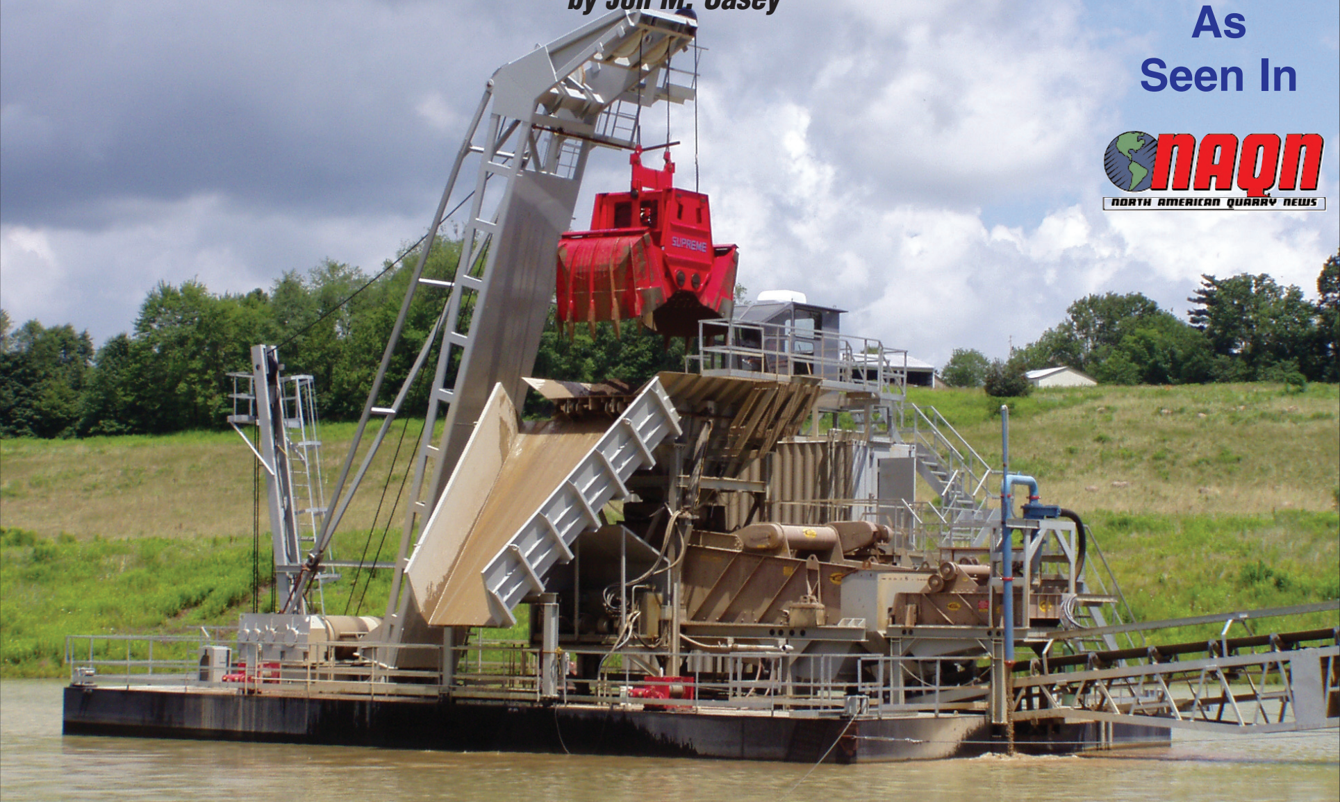
The Supreme Clam Bucket is fully ported with drainage holes that allows excess water to flow back into the lake rather onto the screens.
