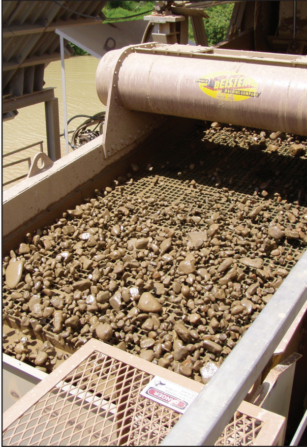
Oversized material is dumped from the grizzly screen, onto the chute and back into the mining pit.
