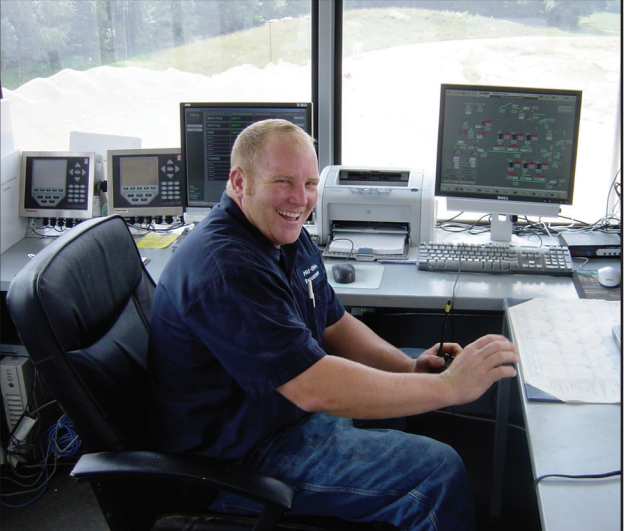
Adam Coleman, plant/scales operator is able to monitor the plant and scales from this location. All components are operated with touch screen controls.
