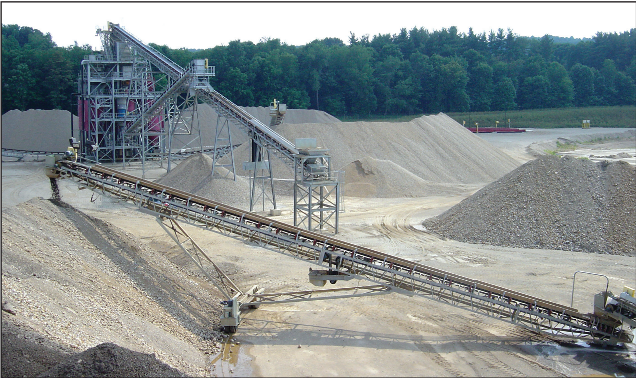
Material can be stockpiled directly from the dredge without the plant needing to operate. This is done with a "buffer" system design, using a radial stacker to either stockpile the material or depositing it onto another conveyor that leads to the processing plant.
