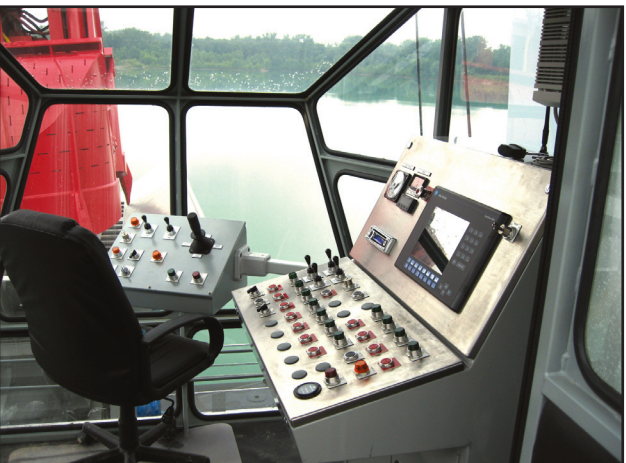
The clean control panel allow the operator an easy view of all the necessary functions of the dredge systems.
