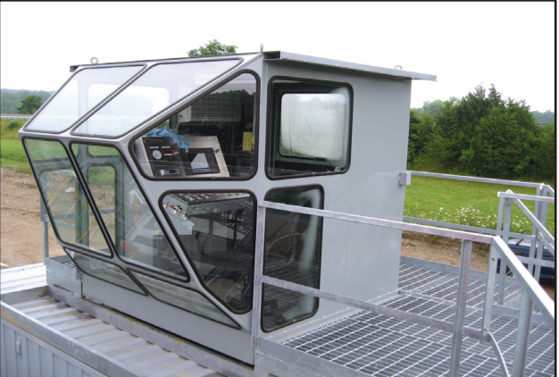
The high visibility cab gives the dredge captain a clear view of all that is going on above and below.
