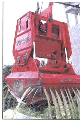
Water drains from the 8-yard, Spade Nose Bucket as it moves into place for dumping. Photos by Jon Casey
