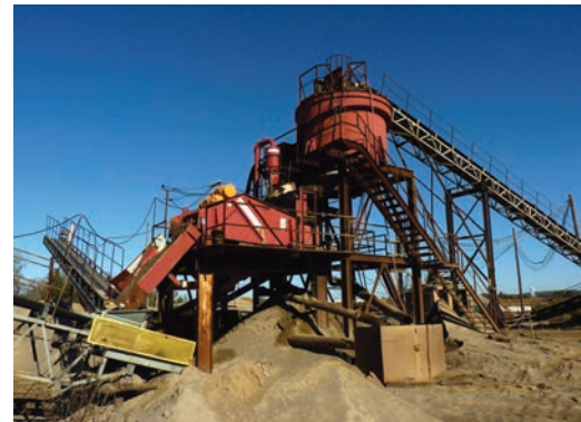
Soehnlens's McLanahan Lites-Out classifier has greatly improved the quality of the company's sand products.
