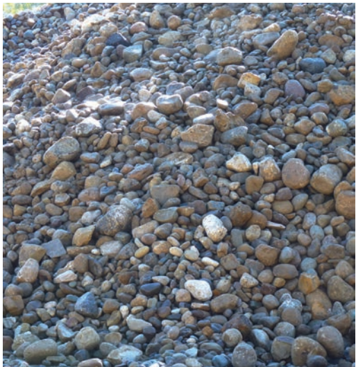
Larger material is set aside to be crushed when there is a sufficient quantity to run a batch of material.
