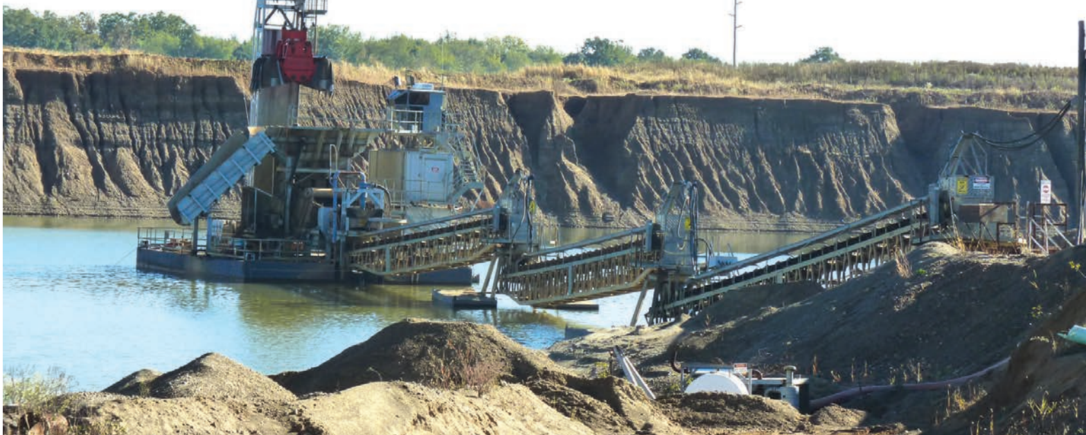
Soehnlén's Supreme, 8-yard clamshell dredge has increased production by helping to more effectively handle the larger, undesirable rocks.
