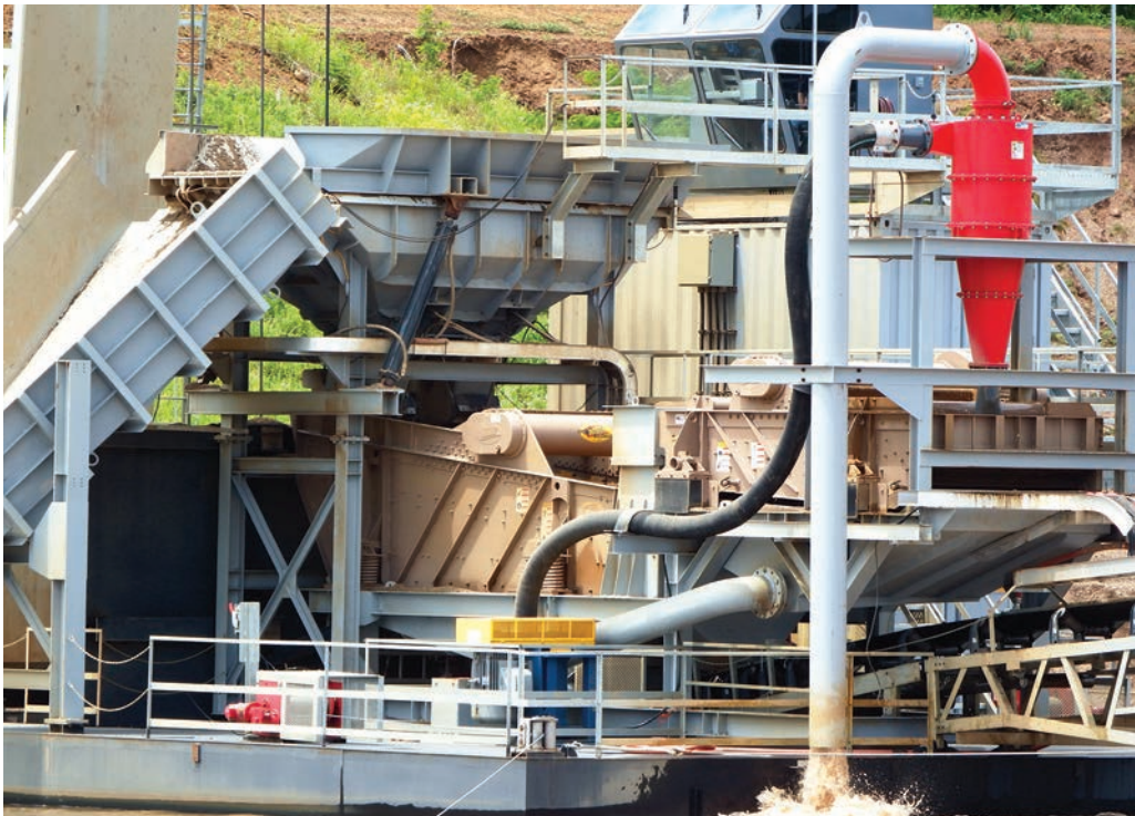
The dredge is outfitted with a 6-foot x 16-foot double deck Deister primary screen, a McLanahan Cyclone and a 7-foot x 12-foot Deister fine recovery screen.
