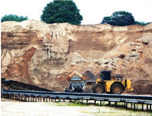
An operator loads material from an area of the quarry face where recent rains have created a washout area.
