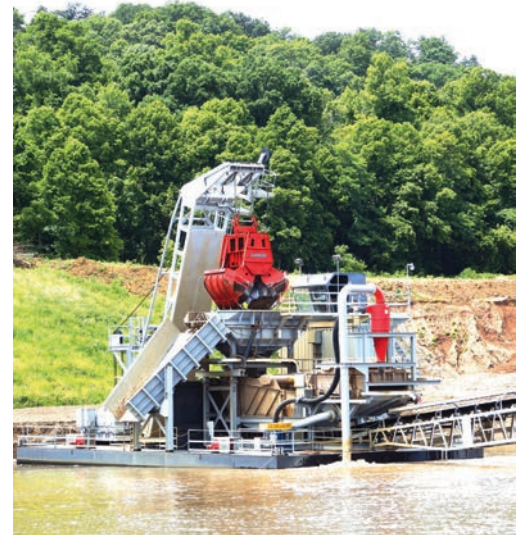
Jaymar, Inc's Supreme Dredge provides a second mining area within the confines of the quarry pit.
