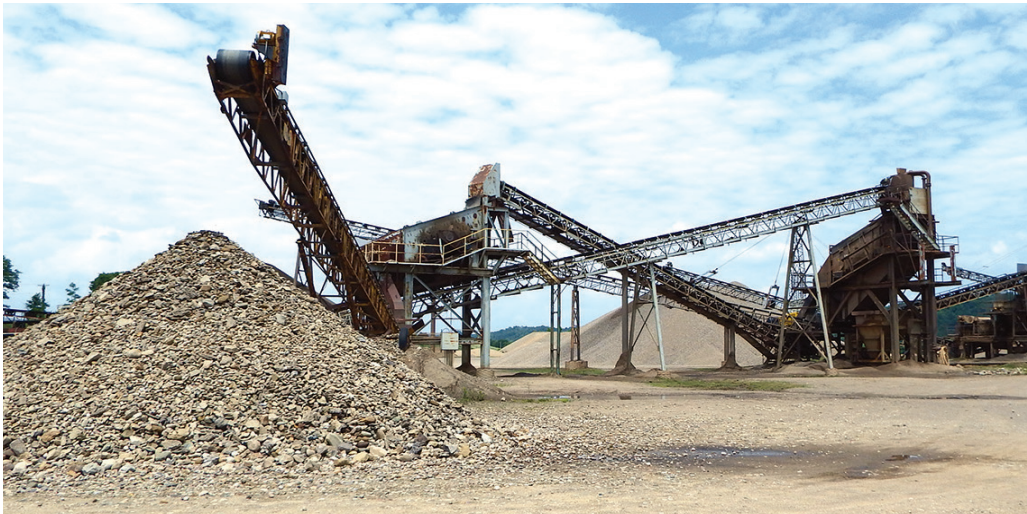
The screen plant provides six products including concrete and masonry sand as well as four classifications of aggregate.
